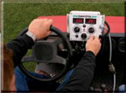
Electric controls with LED readouts and a key start for engine models.
