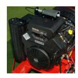
◆ The Agrimeta I Turbine Blower is powered by a **KOHLER 23HP Pro- Command** gas engine.
