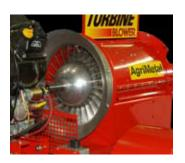
◀ The Agrimeta I Turbine blower marks another chapter in Agrimeta I's long history of Turf Care Products. The new turbine is constructed with an Aluminum Cast **Turbine Propeller, which is electronically** balanced to provide years of trouble free service
