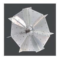
OUR IMPELLERS ARE MADE FROM 6061T6 ALUMINIUM. THEY ARE DYNAMICALLY BALANCED FOR A SMOOTH AND VIBRATION FREE OPERATION. ITS LIGHTWEIGHT CONSTRUCTION REDUCES THE LOAD ON THE BELT AS THE PTO IS ENGAGED. AN ALUMINIUM IMPELLER REQUIRES LESS ENERGY AT FULL THROTTLE.THIS IS WHY OUR BLOWERS DEVELOP SUPERIOR WIND VELOCITY.
