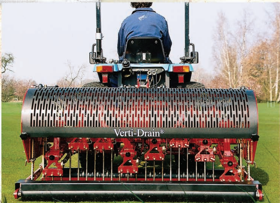
Verti-Drains adjustable parallelogram design shatters the soil, and also allows for clean coring, on all models.
